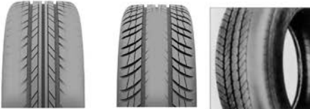
Shoulder wear Intermediate wear One-sided wear
